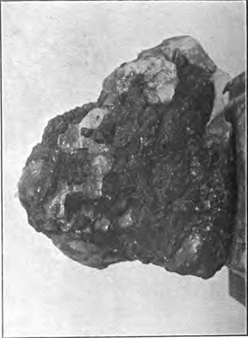
BLOCK OF FLUORSPAR (DARK) INTERGROWN WITH QUARTZ (PALE), FROM MATALE [FARSONS]. Slightly less than one-half natural size.
