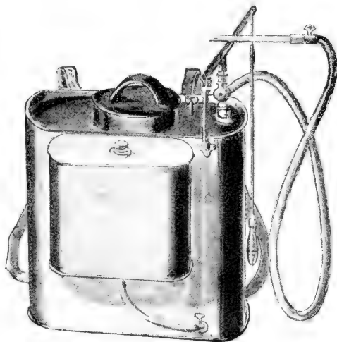
FIG. 17. — An improved form of a kerosene reservoir attached to a knapsack pump.
