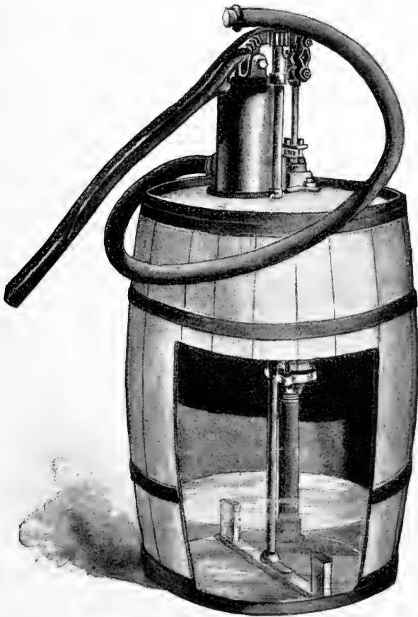
FIG. 29. — Spray pump, with large air chamber; the paddle at the bottom of the barrel acts as an automatic agitator.
