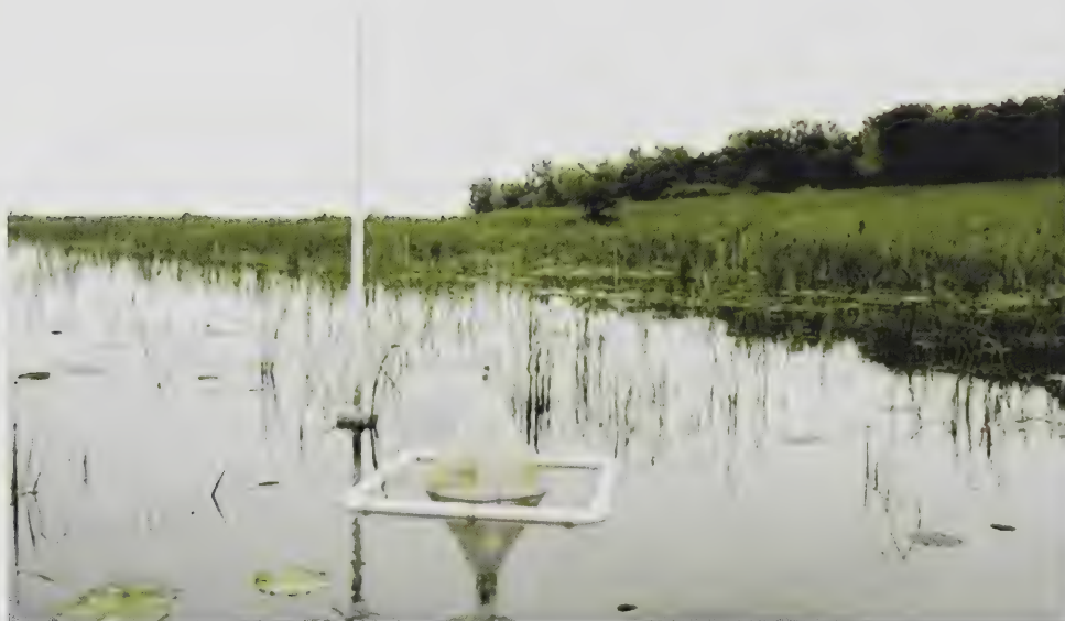
Figure 1. Emergence trap design used to collect adult aquatic insects in Merwin Preserve at Spunky Bottoms. Photo by A. Maria Lemke, The Nature Conservancy.
