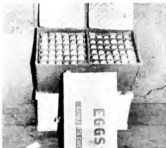
Figure 3 (a). Thin wooden cases, the study showed, often cause trouble because the covers may split and give way.
