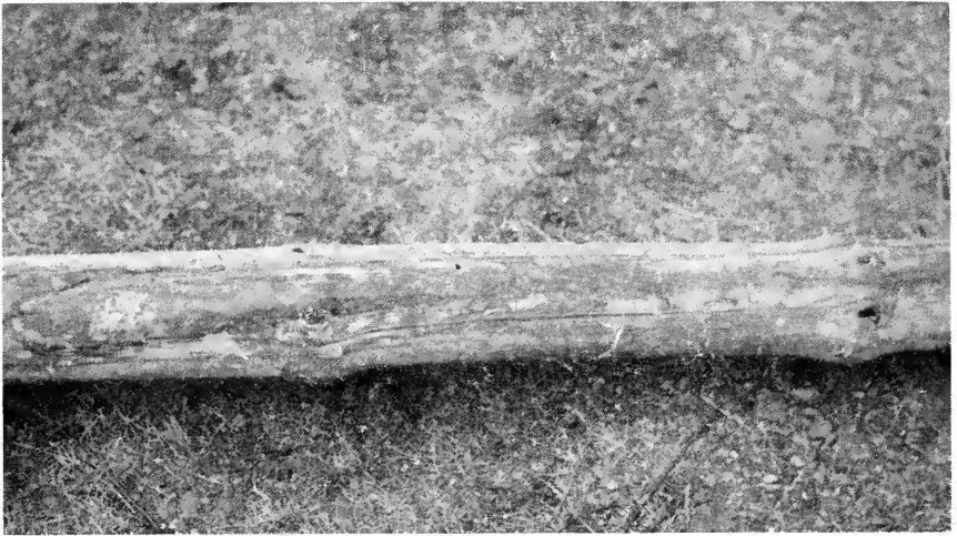
Portion of a pole from a red pine tree treated with sodium arsenite tab seven months earlier. The path of chemical action is seen by the parallel lines on the post.
