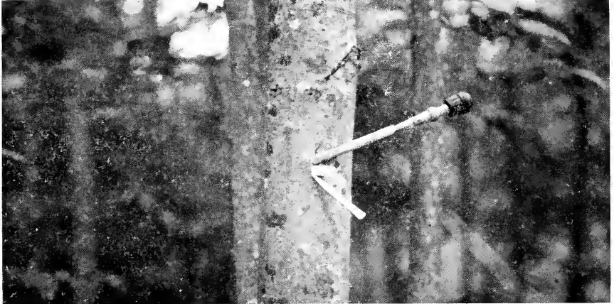
This is the equipment for killing trees with treated tabs. The picture shows the spud, tab, and pointer, with the tab partly inserted in the bark pocket.
