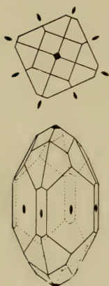
Fig. 12. A Crystal of Zircon showing the Symmetry of Tetragonal Crystals.
