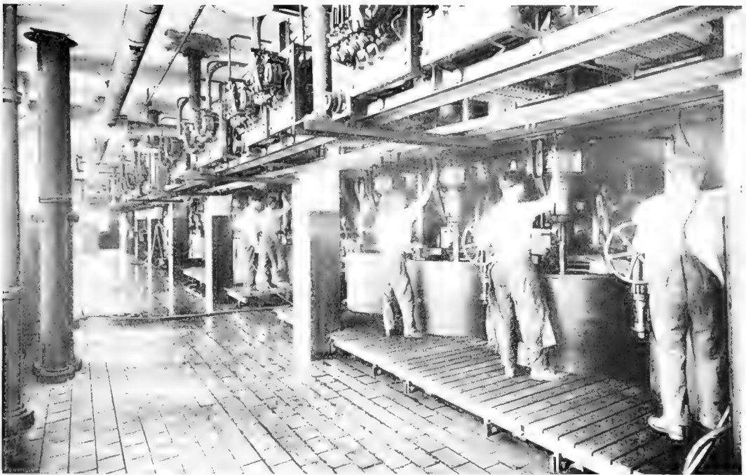
"Purging" the Sugar in the Centrifugals
