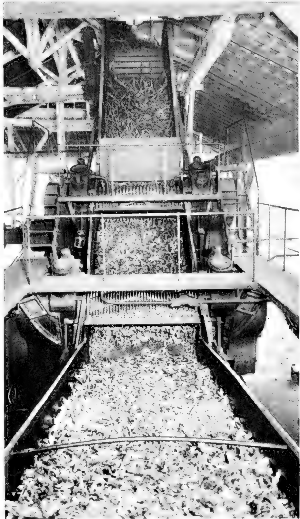
Cane Mat in Foreground Leaving Second Crusher
