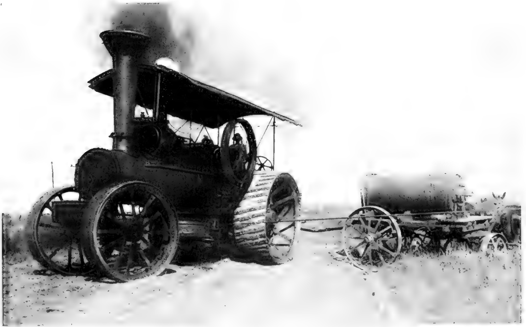
Steam Plow (taking on water) By means of a steel cable the plow or knifer is drawn back and forth
