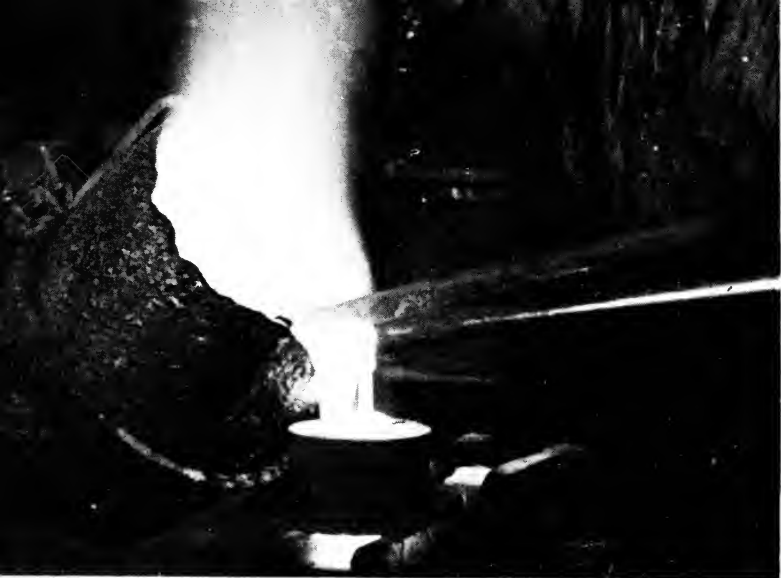
Casting the Capsule's shell in molten Cupaloy
