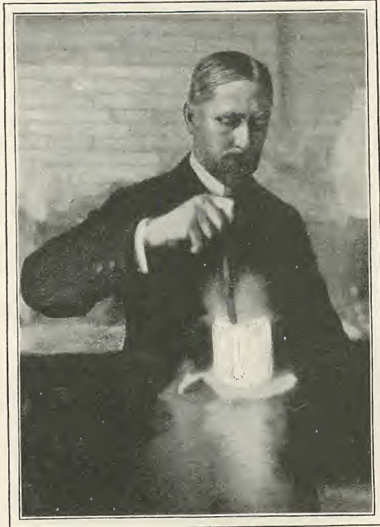
BURNING STEEL IN AN ICE TUMBLER PARTLY FILLED WITH LIQUID AIR. A point of interest in this experiment is the contrast in temperatures; steel is burning at 3,500deg. F. in an ice receptacle containing liquid air at 312deg. below zero.
