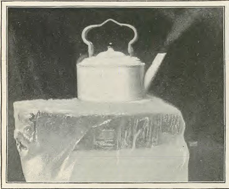
LIQUID AIR BOILING ON A BLOCK OF ICE.
