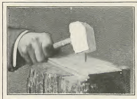
DRIVING A NAIL WITH A HAMMER MADE OF MERCURY FROZEN BY LIQUID AIR.
