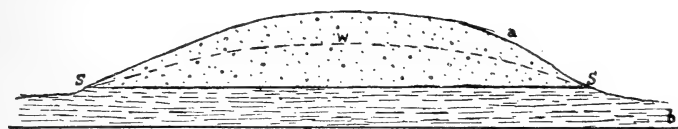
FIG. 126.—HEAPING UP OF WATER IN SUPERFICIAL DEPOSITS.
