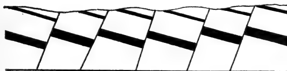
FIG. 46.—STEP-FAULTS HADING AGAINST THE DIP.
