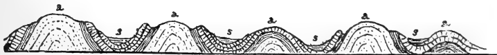
FIG. 139.—SYMMETRICAL FOLDS OF THE JURA MOUNTAINS. a, a, anticlines; s, s, synclines.
