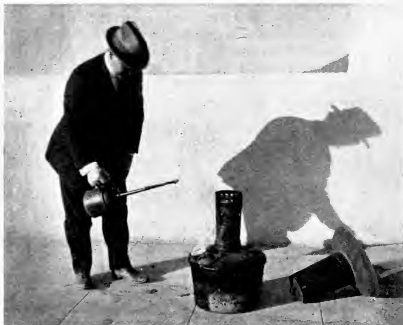
Fig. 9.—Lighting a good recent type of orchard heater by means of a torch containing distillate. The fire being applied to a small amount of excelsior placed in the tube of the down draft. The cover on the right when placed on the heater, extinguishes the fire and excludes rain. Photo by Barrett.
