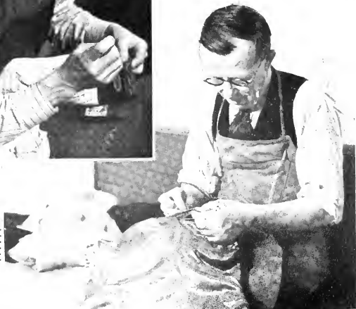
Fig. 5. Here skilled operatives are shown Buttonholing, Felling and Serging.
