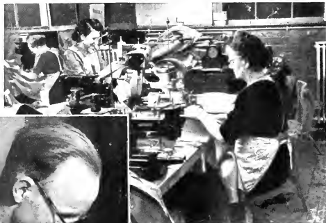
Fig. 5. Here skilled operatives are shown Buttonholing, Felling and Serging.
