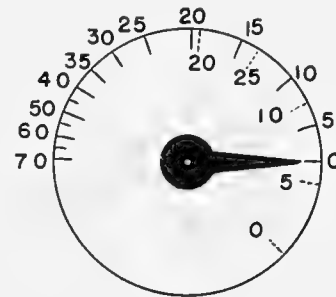
FIGURE 3. Calibration of gain control of an A scope. (Dotted lines are uncorrected calibration.)
