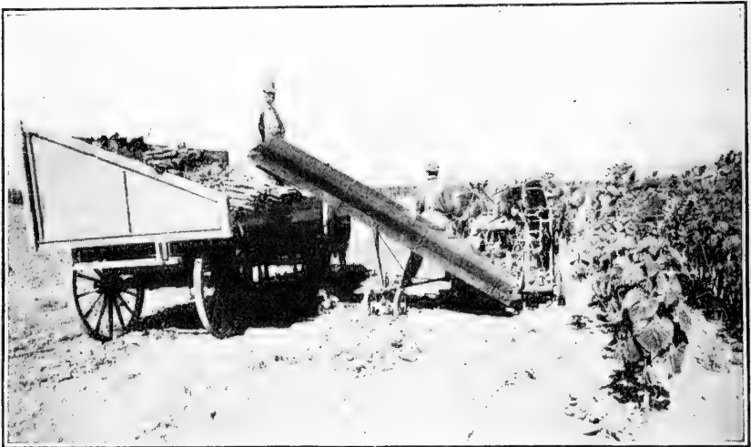
FIG. 3.—Harvesting sunflowers for silage with a row binder equipped with an elevator to carry the bundles directly into a header barge.
