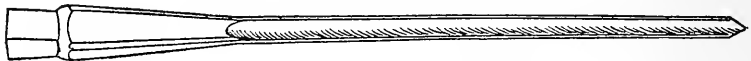
Fig. 12.—Hartley Chisel. This chisel is pointed, V shape on section, and is very convenient for cutting the groove in the bone.
