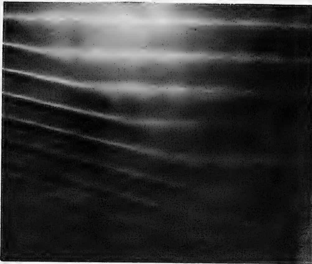
Fig.14 Photograph showing incident, refracted, and reflected waves at the boundary of the step model.
