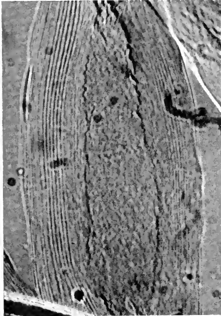
FIG. 4. Longitudinal view of the layers in the secondary wall of a swollen 51-day fiber. Magnification \times 500 .
