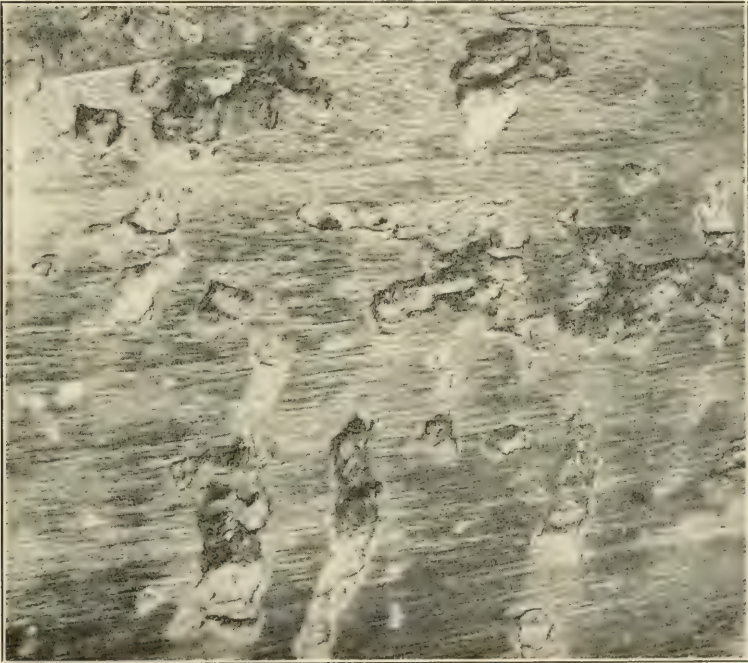
Fig. 58.—Portion of a slab of cottonwood, showing the effect of a wood-destroying fungus ( Elfvigia megaloma ). Original.
