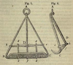
To have a clear idea of the dredge, and the parts which compose it, we must imagine a circular bar of iron, forged in the shape of an almost equilateral triangle, A, B, C, of the above figure, whose two extremities are joined at A. To form the summit or point of the triangle, each of the sides should be above five feet. The two branches, AB, and AC, are rounded and bent, as they approach the base of the triangle. The base, BC, is forged into a plate, six inches in breadth with a sharp
