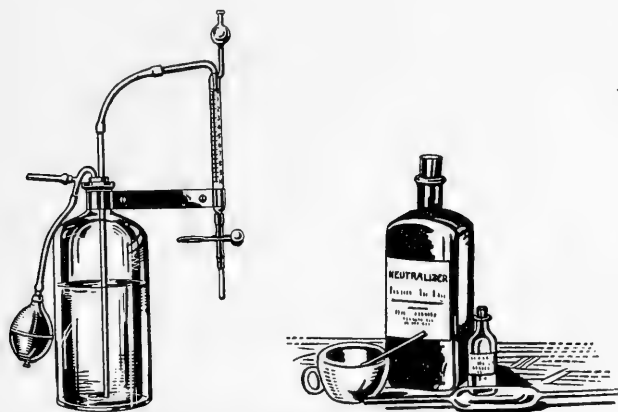
Fig. 148. Troy Salt Test Apparatus.
