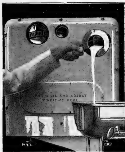
Fig. 108. Emptying Overrun Cup Into Freezer Hopper.
