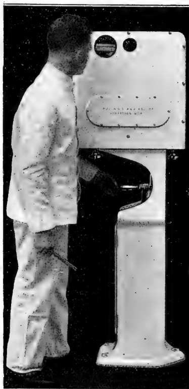
Fig. 112. Making Reading for Overrun.
