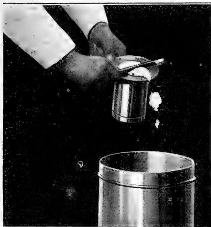
Fig. 111. Scraping Overrun Cup Level Full of Ice Cream.
