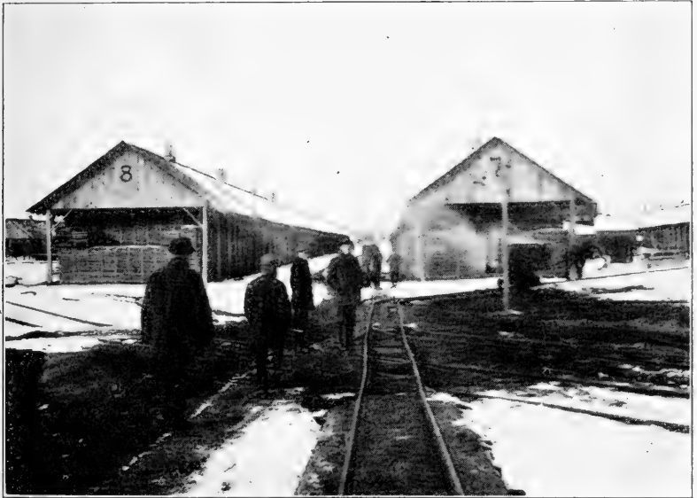
Steaming staves being rolled out on trucks and piled under sheds. Over 50,000,000 staves are made annually in New York for slack cooperage used in the shipment of apples and other fruit, cement, vegetables, crockery, sugar, flour, etc. The principal woods used are birch, beech, maple, elm, spruce and ash. Photograph taken at the plant of the Brooklyn Cooperage Co. at Faust, N. Y.
