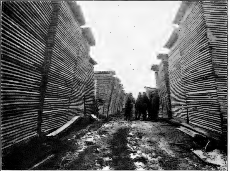
Hardwood lumber, chiefly hard maple, yellow birch, beech, elm and basswood seasoning in the yard preparatory to being sent to the many wood-using industries of the State for further manufacture into flooring, furniture, implements, machinery, boat building, instruments and a great many other wood products. We should grow all of the wood used in the State, instead of sending over $60,000,000 to other States for this material every year.
