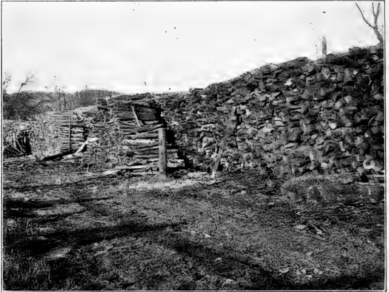
Wood yard of the Maryland Wood Products Co. at Maryland, Otsego county, showing the character of limb and body wood, chiefly beech, birch and maple. This wood is seasoned from one to two years before being run into the ovens and made into charcoal, wood alcohol and acetate of lime. Photograph by NELSON C. BROWN.
