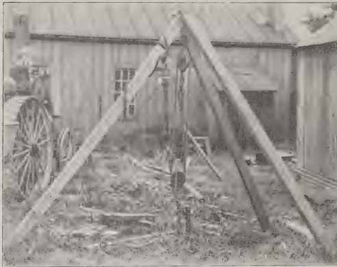
TESTING BULL DOG GUY ANCHOR.
