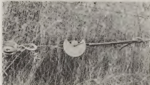
The Dynamometer Measuring the Strain Put Upon the Cedar Poles in Testing Them to the Breaking Point to Determine Their Strength.
