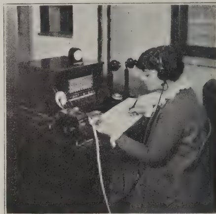
Central Machine Switching Cutover—Service Observing Desk.
