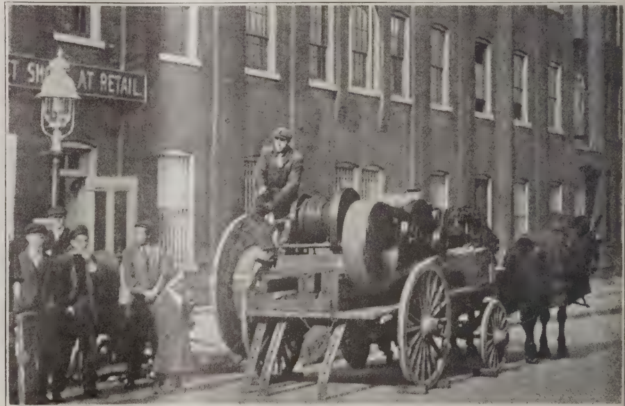
Fig. 16. Old Type Gasoline Engine Driven Winch on Horse-Drawn Truck.
