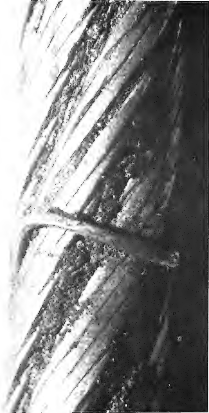
Figure 21. Wire rope 1-1/2-inch in diameter with 12% crown wire wear.
