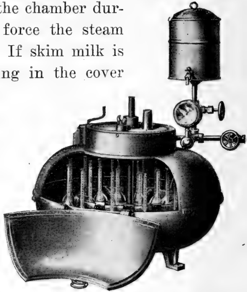
FIG. 23. Type of Babcock steam turbine testers.
