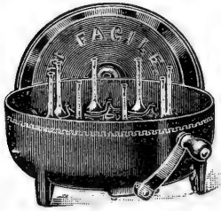
FIG. 20. Type of Babcock hand testers.
