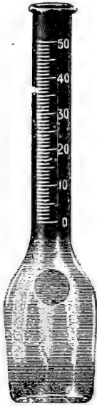
FIG. 33. The 50% cream test bottle.
