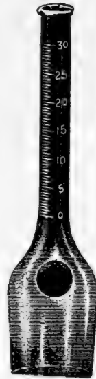
FIG. 32. The 30% cream test bottle.
