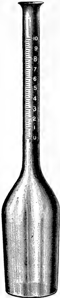
FIG. 5. Babcock milk test bottle.
