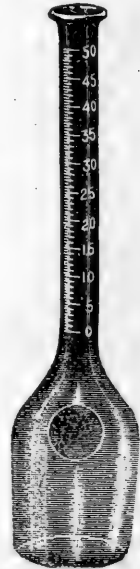
FIG. 33a. The 50% 9 gram cream test bottle.
