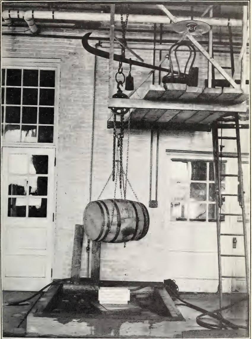
METHOD OF TEST—SIDE DROP.
