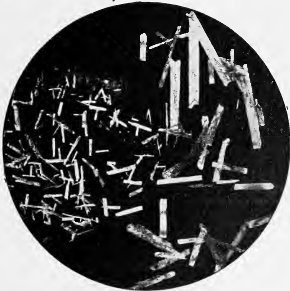
FIG. 150. Caffeine gold chloride; crystals formed on the addition of a solution of gold chloride to a dilute aqueous solution of caffeine.
