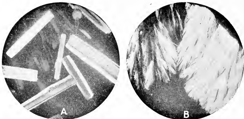
FIG. 149. Orthorhombic crystals of Mannitol (Mannit) obtained from aqueous solutions: A, large crystals; B, feathery aggregates of needles.
