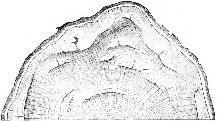
FIG. 159.—Transverse section of an oak-stem showing numerous sun-cracks. One half natural size.
