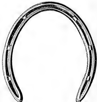
A hind running plate, ground-surface.
