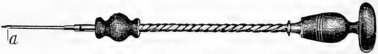
Spiral drill for boring the hole into which a round wire nail is driven to fasten a toe-crack. ( a ) three sided point of drill (similar to the point of a stilet of a caecal trocar).
