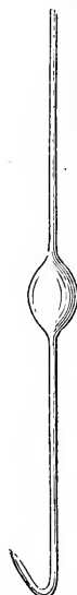
FIG. 50. PIPETTE WITH BULB, FOR INTRODUCING LIQUID REAGENTS INTO ABSORPTION TUBES STANDING OVER MERCURY. (Scale about \frac{1}{2} .)
