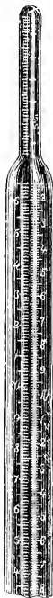
FIG. 47. ABSORPTION TUBE 1 , WITH DOUBLE SCALE, AS MADE BY ALVERGNIAT. (Scale about \frac{1}{2} .)
