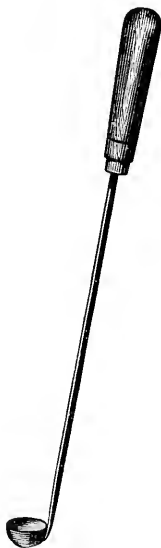
FIG. 48. IRON SPOON EMPLOYED IN TRANSFERRING TUBES FROM ONE MERCURIAL TROUGH TO ANOTHER. (Scale about \frac{1}{2} .)
