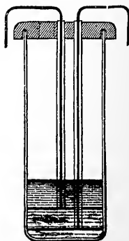
FIG. 29. Conductivity cell for poor conductors or small quantities.
