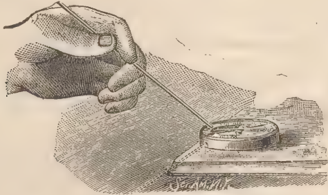
Fig. 1. MAGNETISM BY INDUCTION FROM THE EARTH.
