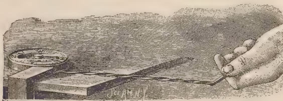
Fig. 2. DEVELOPMENT OF MAGNETISM BY TORSION.
