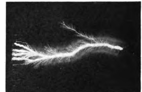
FIG. 10.—A DISCHARGE FROM A NEGATIVE POLE WITH THE PLATE AS THE POSITIVE
