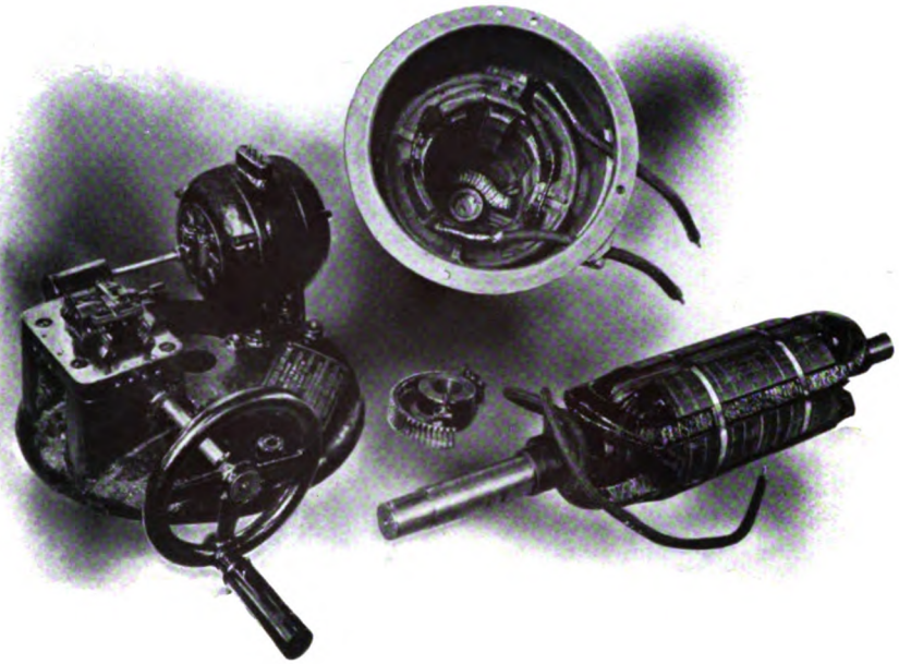
FIG. 15.—PARTS OF AN INDUCTION REGULATOR
