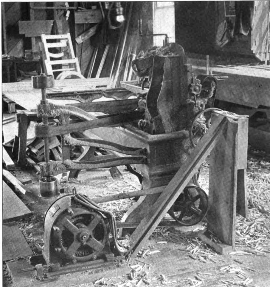
A 2-H. P. WESTINGHOUSE INDUCTION MOTOR DRIVING A TENONING MACHINE
