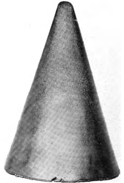
FIG. 3.—A CONE ON WHICH COPPER HAS BEEN DEPOSITED WHILE THE CONE IS ROTATING. THE EFFECT OF THE DIFFERENT PERIPHERAL SPEEDS IS CLEARLY SHOWN
