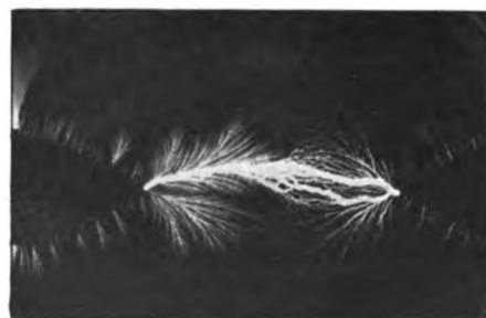
FIG. 8.—A DISCHARGE BETWEEN TWO POLES, THE NEGATIVE BEING AT THE LEFT AND THE POSITIVE AT THE RIGHT
