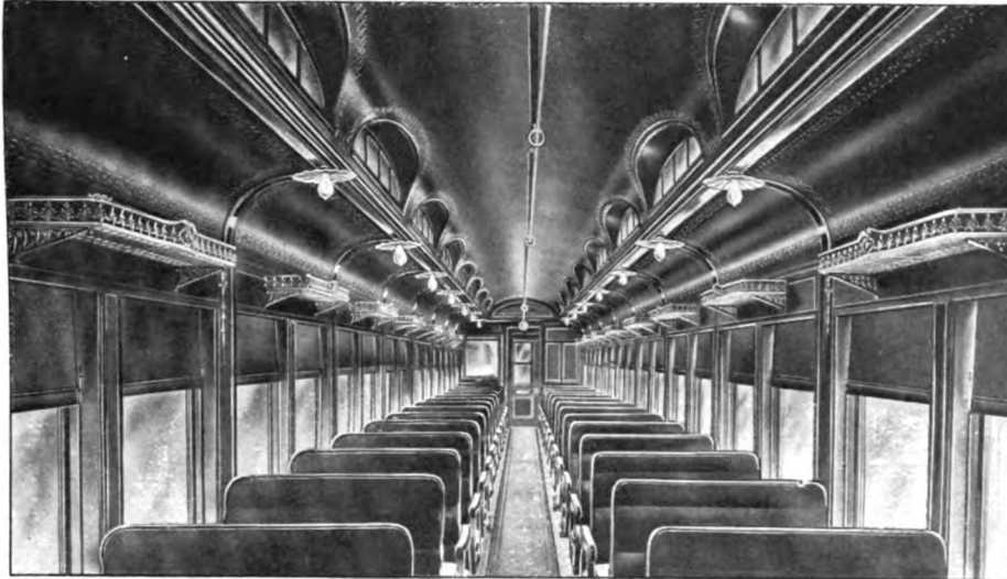
FIG. 20.—AN "EMPIRE STATE EXPRESS" CAR ON THE NEW YORK CENTRAL & HUDSON RIVER RAILROAD LIGHTED BY THE MOSKOWITZ SYSTEM
