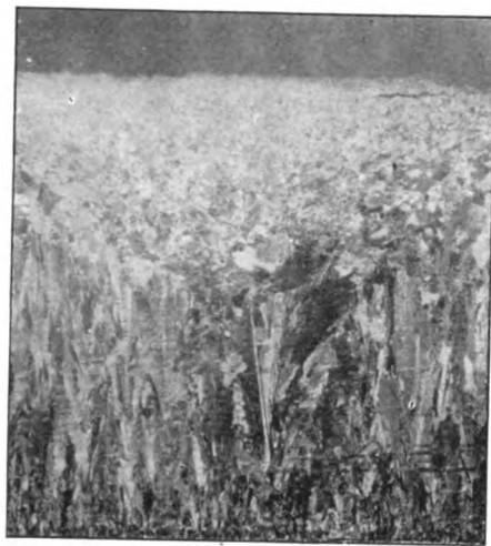
FIG. 17.—A MICROGRAPH OF DEPOSITED COPPER
