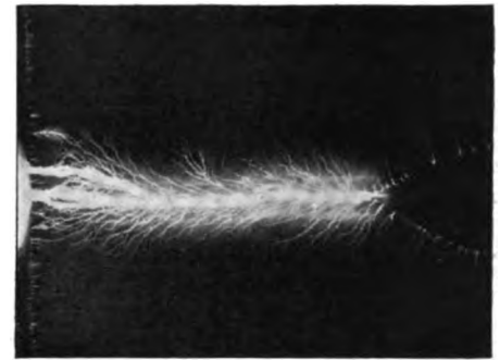
FIG. 9.—A DISCHARGE FROM A POSITIVE POLE WITH THE PLATE AS THE NEGATIVE
