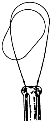
FIG. 1.—A BROKEN FILAMENT OF A HELION LAMP WHICH FUSED AGAIN WHERE THE PARTS CAME IN CONTACT
