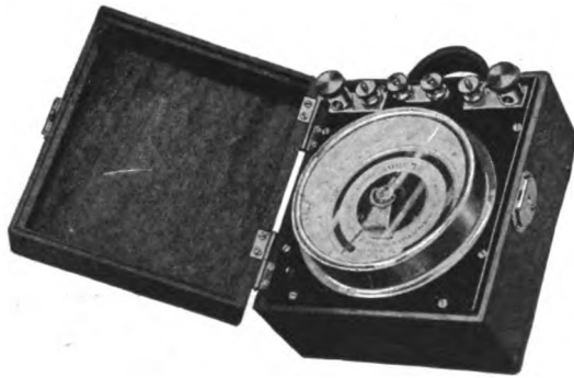
FIG. 4.—DIRECT-SWING TYPE OF METER.
