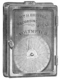
FIG. I .- RECORDING MILLI-VOLTMETER.
