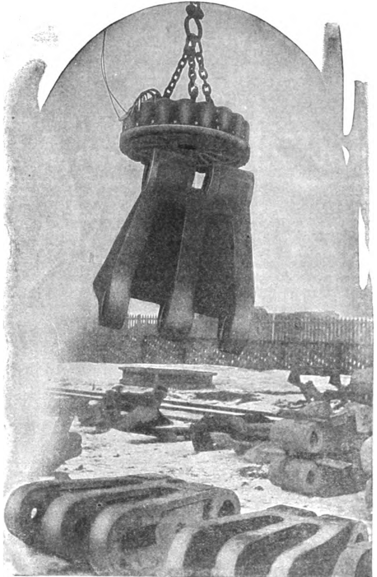
36-INCH MAGNET, HANDLING HEAVY CASTINGS. THE CRANE OPERATOR CAN PERFORM WORK OF THIS SORT WITHOUT THE ASSISTANCE OF GROUND MEN. THERE IS NO HOISTING TACKLE TO BE ADJUSTED
