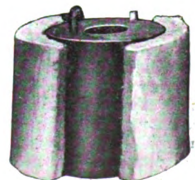
Metal Block with Magnesia Insulation
