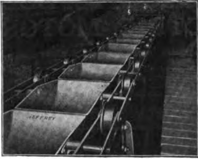
Jeffrey Overlapping Pivoted Bucket Carrier, Passing Over Coal Bunkers
