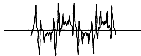
FIG. 37.—OSCILLOGRAM OF CURRENT CURVE PRODUCED BY SAME VOLTAGE WAVE IN CIRCUIT CONTAINING CAPACITY.
