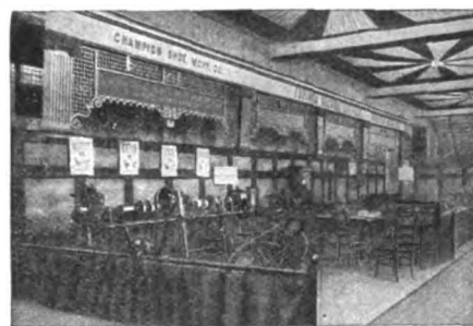
CHAMPION SHOE-REPAIRING OUTFIT DIRECT-DRIVEN BY WESTERN ELECTRIC MOTOR.
