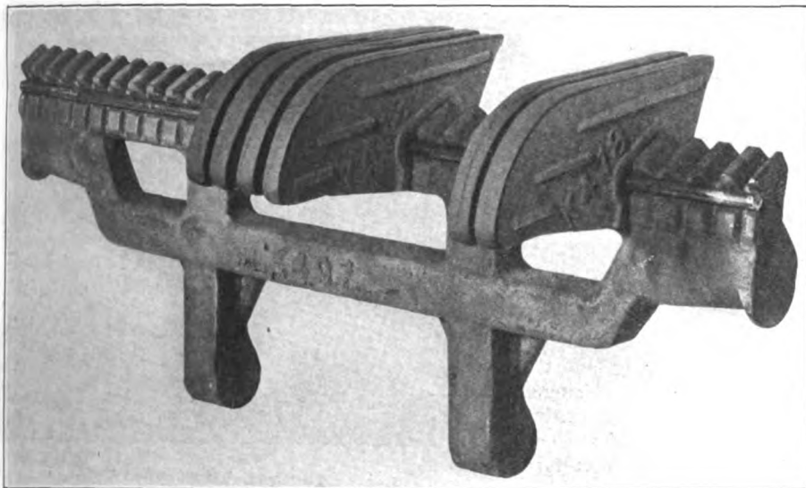
UPPER GRATE BARS, NEW MODEL WESTINGHOUSE RONEY MECHANICAL STOKER.
