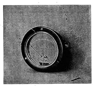
Flush Type Direct-Current Voltmeter.
