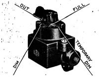
Switch for Convenient Control of Locomotive Headlight Through Several Degrees of Intensity.
