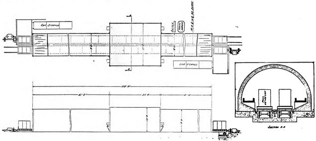
Fig. 3.—Continuous Recuperative Cary Type Furnace for Annealing Tin Plate, Cold-rolled Steel, Etc.
