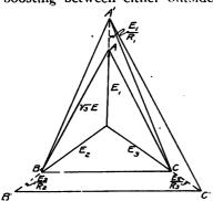
4.-Y-Connected Three-Phase Network with One Phase Boosted.
