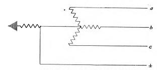
Fig. 2.—Diagram Showing Location of Resistor With Respect to Station Transformer Bank, Neutral Conductor and Transformer Neutral Point and Earth.
