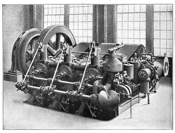
Triplex Diesel Type Oil Engine.
