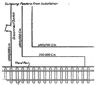
Schematic Layout of Railway Feeders for Changing Equivalent Feeder Length With Load.
