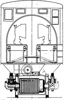
Fig. 2.—End Outline and Motor Cross Section of New Gearless Locomotive.
