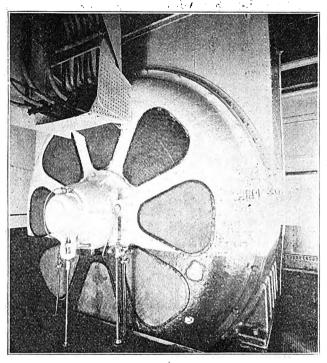
Forward End of One of the Four 7000-hp. Propeller Motors of Battleship New Mexico. Diameter of Motor is 12 ft.
