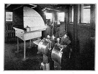
Navigating Bridge with Steering Control and Electric Apparatus for Transmitting Signals to Engine Rooms.
