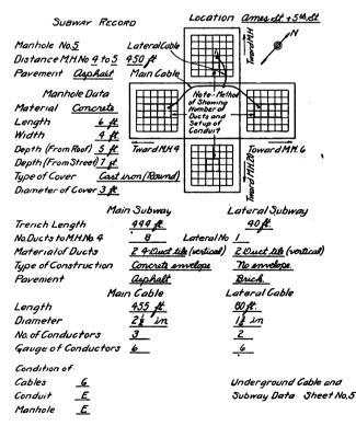
Fig. 4.—Sample Field Sheet for Recording Underground Cable and Subway Data.
