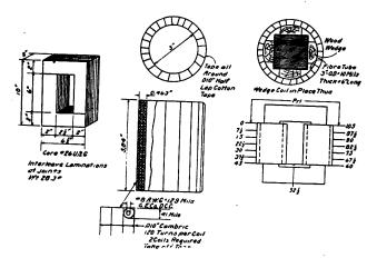
No. 464.—Design of Autotransformer with Numerous Taps.
