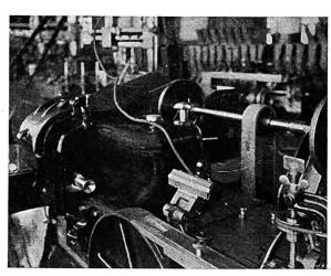
Near View of the Electric Heater Swung Up for Inspection.
