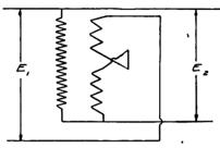
Fig. 8.—Single-Phase Choking Set with Secondary Colls in Series.
