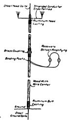
Tool for Locating Defective Pin-Type Insulators Supported Upon-Nonmetallic Structures.
