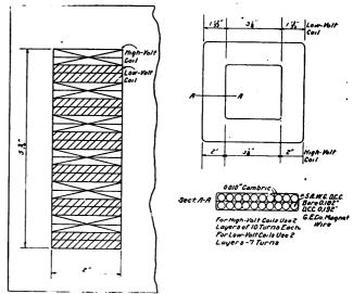
No. 472.—Rewinding of a Transformer.
