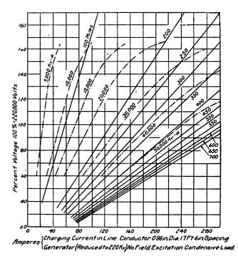
Fig. 4.—Generator and Line Characteristics: 60-Cycles, 220,000 Volts, Generators With Short Circuit Ratio 1.5.
