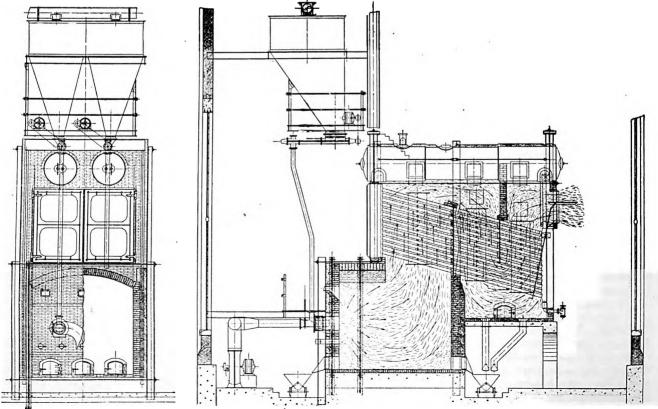
Fig. 3.—500-Hp. Babcock and Wilcox Boller Arranged to Be Fired with Pulverized Coal.
