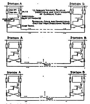
Figs. 6, 7 and 8.—Balanced Protection for Two Parallel Lines (Discriminating).
