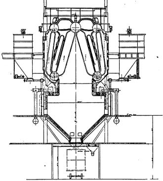
Fig. 1.—2400-Hp. Detroit Edison Type Boller Arranged to Burn Pulverized Coal at 200% Rating.
