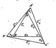
Fig. 6.—General Case of a Delta Three-Phase Booster with Unequal Boosting of Each Phase,
