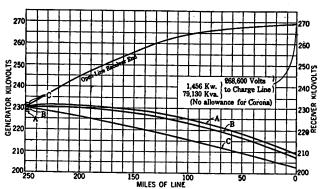
Fig. 3-220-kv. Transmission Line Characteristics-Relation Between kw., kv., p f. and Condenser kv-a.-Conductor-450,000 cm. Copper-308,200 Steel.
