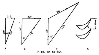
blades, 218 ft. per sec. in direction at right angles to direction of rotation. Fig. 1B shows a similar condition giving maximum obtainable efficiency employing a 35 deg. blade angle and Fig. 1c a condition in which the steam speed is 100% greater than the blade speed.
