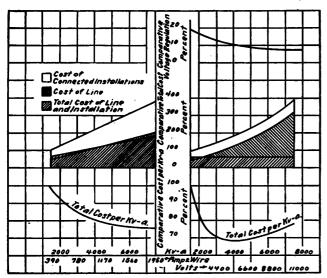
Fig. 2.—Relative Costs and Voltage Regulations for Increasing Capacity Including Lines, Connected Installations and Substations.
