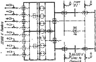
Single-Line Diagram of North Substation—Dotted Lines Show Future Extensions,
