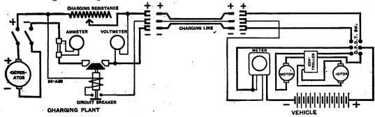
Wiring Diagram of Typical Installation of Automatic Charge-Controlling Ampere-Hour Meter of Battery Trunk, Showing Circuit-Breaker on Charging Panel Controlled by Meter Contact at Full Charge Point.
