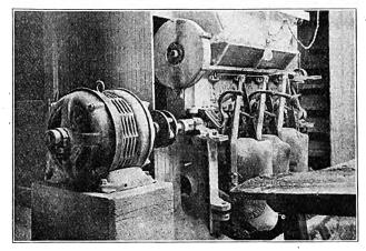
Fig. 2.—15-hp., 1140-r.p.m. Westinghouse Motor Driving Sacking
