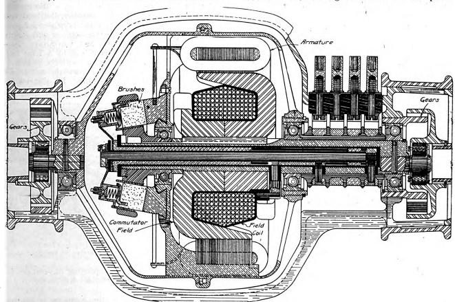
Diagram Showing Arrangement of Motor Parts and Gears.
