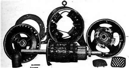
Type "E," 25-hp., 230-Watt, 1150-r. p. m. Motor Dismantled.
