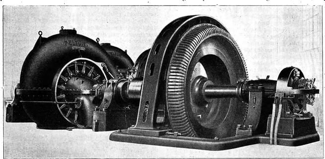
Pelton Water Wheel Driving Canadian General Electric 3750-kv -a., 2300-volt at 350 r.p.m. at Plant of Pacific Mills, Ltd., Ocean Falls, B. C.
