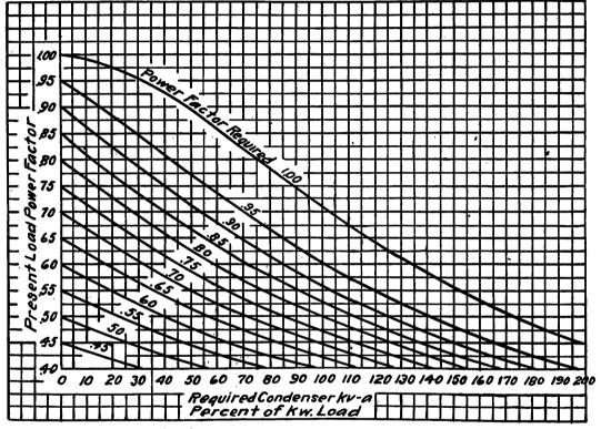
Fig. 6.—Curves Showing Condenser Kv-a. Required for Any Desired Power-Factor Correction in Per Cent of Existing Kilowatt Load.
