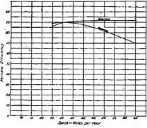
Fig. 3.—Comparative Efficiency Curves of Geared and Gearless Locomotives.
