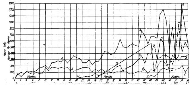
Fig. 4.—Curves Showing Variation of Lamp Life with Time for Five Different Makes of Lamps.
