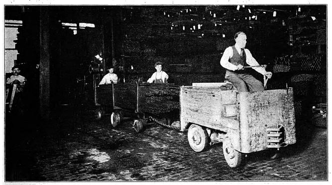
For Hauling Materials From the Stock or Receiving Rooms to the Machines the Electric Industrial Tractor Offers Many Advantages.
