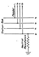
Fig. 1.—Diagram Showing Station Bus, One Four-Wire Feeder and Earthing Resistor.
