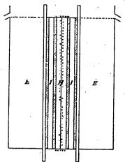
Thermal Unit Used for Determining Thermal Conductivities.
