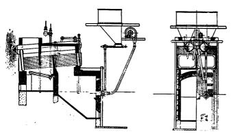
Fig. 2.-425-Hp. Heine Boiler Arranged for Pulverized-Coal Firing.
