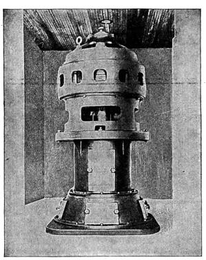
Centrifugal Water Pump Driven by 200-hp. Vertical Induction Motor at Savannah Water Works.
