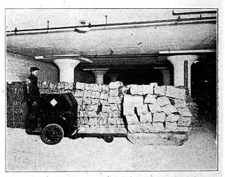
The Electric Lift Truck Can Also Be Used in Distributing Within the Warehouse if the Material Can Be Loaded on Skids.
