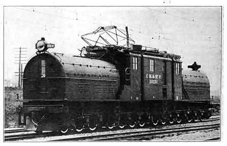
Fig. 1.—3000-Volt, Direct-Current, Gearless Passenger Locomotive for C., M. & St. P. Cascade Electrified Zone.
