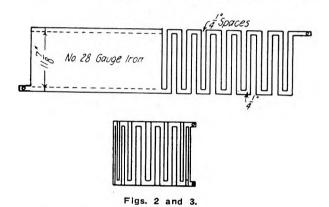
black iron sheet 11% ins. wide and of such length as to encircle the bushing, this sheeting being cut into the form shown in Fig. 2.
