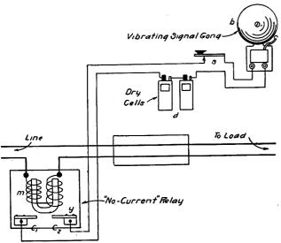
Wiring Diagram for Audible Signal.
