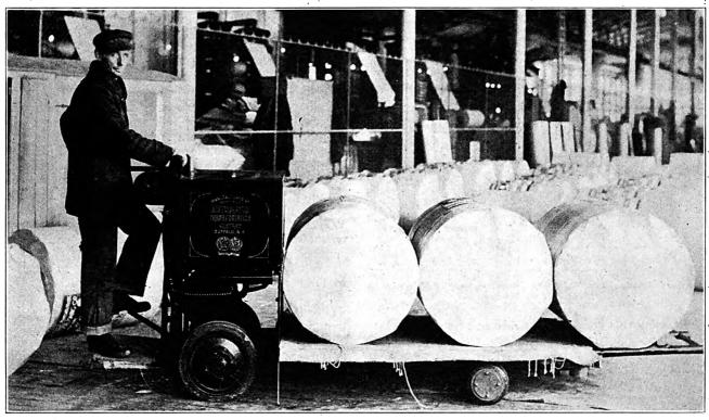
Paper Rolls Are Difficult and Dangerous to Handle by Hand-The Electric Truck Handles Them Easily, Quickly and Safely.
