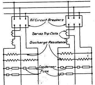
Fig. 3.—Elementary Diagram of Static Condenser Installed on Three-Phase Circuits.
