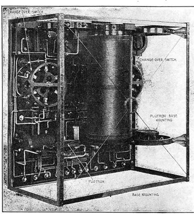
Fig. 5.—Rear View of the Set After Pliotrons Have Been Removed.
