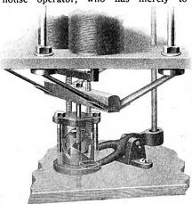
Fig. 3.—Contact Mechanism With Fluctuation Compensator and Special Locking Device.
