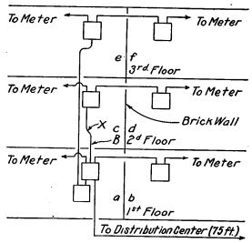
Wiring Diagram Showing Location of Circuits and Fault.
