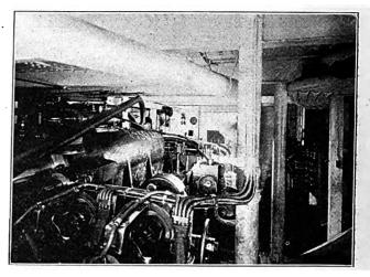
View of Steering Apparatus (Chiefly Electrical) Looking Forward-Note Two Motors in Foreground.
