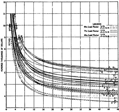
Fig. 4—Economic Comparison of 200 kv. Transmission Conductors—Annual Cost Curves—250 Miles, 100,000 kw. Single Circuit Line. (See table for explanatory data.)
