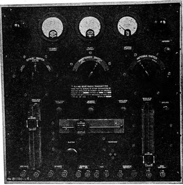
Fig. 3.—Front View of Marconi Wireless Set Used in Seaplanes.
