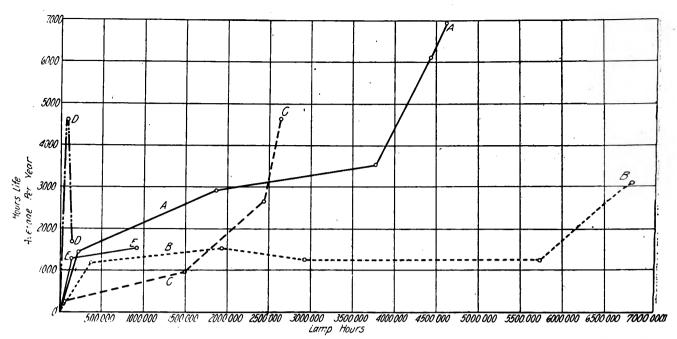
Fig. 5.-Curves Showing Variation of Lamp Life with increase in Lamp-Hours.
