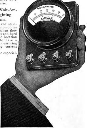
"Handy" Volt-ammeter for Automobile Testing.
