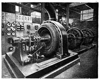
Motor End of Pump Unit Showing General Electric 1800-Hp.
