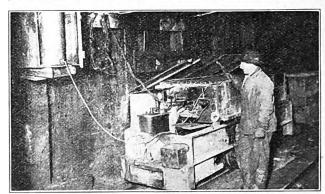
Fig. 2.—Charging and Watering Station on 13th Level of an Idaho Mine—A 31/2-ton Battery Locomotive Is Being Charged.
