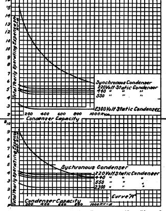
Fig. 4.—Total Yearly Operating Expense per Kv-a./Kv-a. Capacity on Basis of Fuli-Load Operation 7000 Hrs. per Year.
