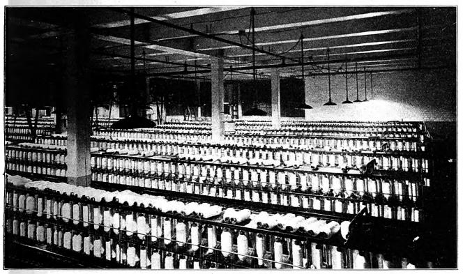
Fig. 1.—Night View in a Spinning Room, Showing General Illumination Meeting All Requirements—Fixtures Can Be Easily Taken
