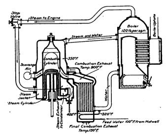
Fig. 1.—Schematic Diagram of the Still Engine.
