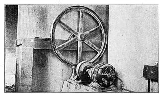
Fig. 6.—7½-hp., 10-pole, 680-r.p.m. Westinghouse Motor Driving Sack Cleaner Through Foote Reducer.
