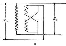
Choking Transformer with Secondary Colis in Parallel.
