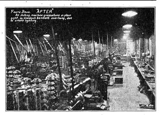
Foote Bros. Gear Works After Lighting Was Rehabilitated— Milling-Machine Graduations in Plain Sight—No Dense Shadows—All Floor Space Utilized.
