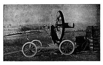
Fig. 2.—An Early Model of the 60-in. Open Type Medium-Intensity Searchlight Adopted for Army Use—This and Later Types Were Much Lighter, More Portable and More Powerful Than the Type Shown in Fig. 1.
