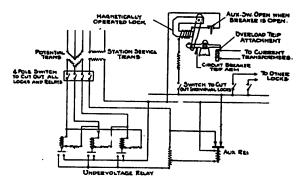
Fig. 15.—Undervoltage and Overcurrent Relay-Scheme of Connections,
