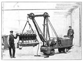
Electric Truck Equipped With Crane for Handling Heavy Material.
