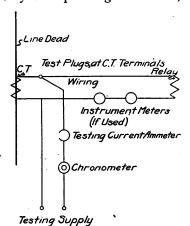
Fig. 1.—Diagram of Connections for Supplying Testing Current to Secondary Terminals of Current Transformer.
