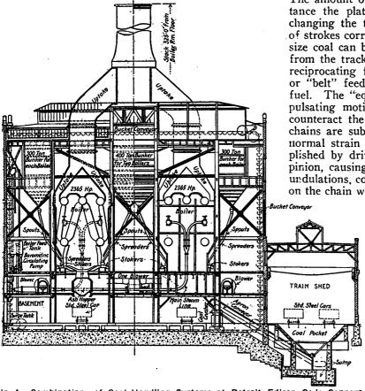
Fig. 1.—Combination of Coal-Handling Systems at Detroit Edison Co.'s Connors
