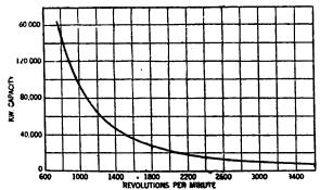
Fig. 3.—Limits of Capacity of Steam Turbines With Double-Flow Low-Pressure Stages.
