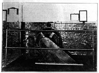
Fig. 7.—One of the Motors Connected to Drive a Group of Machines Through Silent-Chain Belt Drive.
