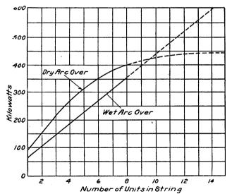
Fig. 2—Typical 60-Cycle Arc-Over Characteristics of Suspension Insulators.
