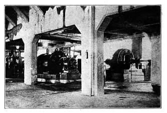
Three 300-hp., 2300-voit Motors Direct Connected to Paper Machine Jordans.
