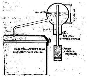
Fig. 7.—Diagrammatic Sketch of Oil Conservator Connected to Transformer Tank.
