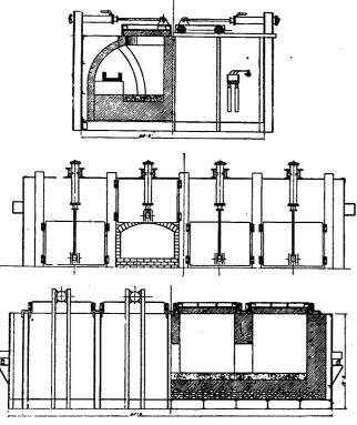
Fig. 1.—Pit Type Furnace for Soaking Ingots for Heavy Forgings and Shafts.
