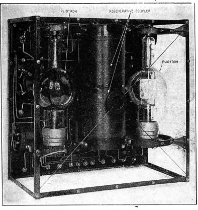
Fig. 4.—Rear View of the Transmitting Set With Pliotrons in Place.
