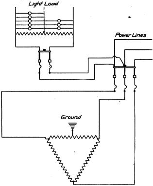
Diagram Showing Method of Connecting Autotransformer in 3-phase Power System.
