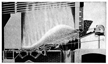
Fig. 4.—Cross-Section Showing Fuel Bed With Underfeed Stoker.
