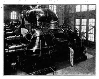
Fig. 4.—Governor and Controlling Mechanism for 70,000-kw.
