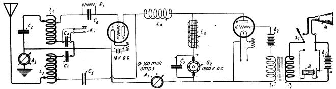
Fig. 1.—Fundamental Circuits of the Wireless Telephone Transmitter for Seaplanes.
