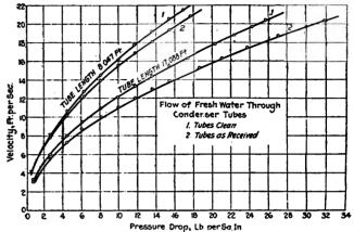
Curves Showing Effect of Tubes as Received From the Factory and Cleaned Tubes Upon Flow of Water.
