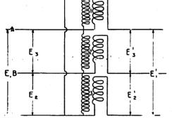
Fig. 5.—Connections of a Simple Delta-Connected Three-Phase Booster.
