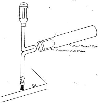
A Handy Method of Applying Extra Power to an Ordinary Screw Driver.
