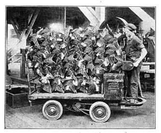
The Elevating Platform Truck is Used Extensively for All Kinds of Handling in and Around Machine Shops.
