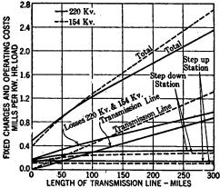
Fig. 1—Economic Comparison of 154-kv. and 220-kv. Transmission—Fixed Charges and Operating Costs—Seven Lines 154 kv. and Four Lines 220 kv.—500,000 kw. Delivered.
