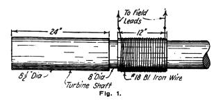
current. A current of about 60 amperes was found sufficient to expand the bushing enough to allow its being forced upon the shaft with a press made of two small screw jacks.
