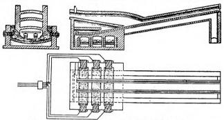
Fig. 2.—Continuous Type Reheating Furnace.
