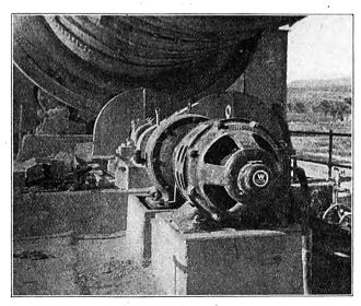
Fig. 4.—50-hp., 440-volt, 60-cycle, 3-phase, 700-r.p.m. Motor Driving Rotary Kiln Through Foote 14 to 1 Reducer; Speed, 1 r.p.m.; Double Reduction, 48 to 1.
