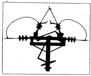
Fig. 2.—Same Switch Partly Opened with Auxiliary Contacts Ready to Open.
