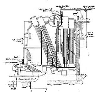
a boiler room comprising 14 Bigelow-Hornsby boilers of 625 b-hp. equipped with Diamond soot blowers and fired by Taylor stokers.
