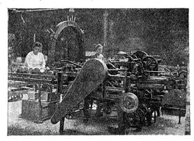
Automatic Box Sealer Driven by 2-hp. Motor.
