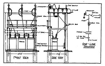
Fig. 5.—Typical Single Circuit Outdoor Substation with Large Capacity Transformers at Ground Level.
