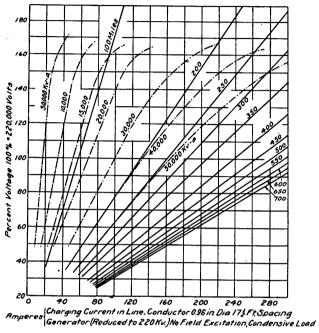
Fig. 3.—Generator and Line Characteristics: 60 Cycles, 220,000 Volts, Generators With Short Circuit Ratio 1.0.
