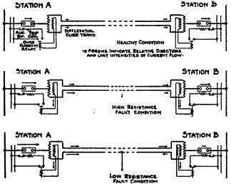
Figs. 11, 12 and 13.—Spilt-Conductor System Protection.
