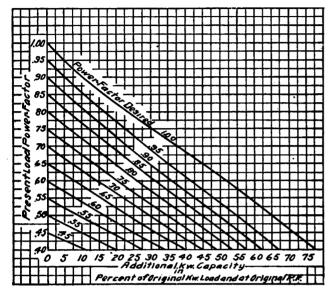
Fig. 7.—Curves Showing Additional Kilowatt Capacity Made Available by a Given Correction of Existing Power Factor.
