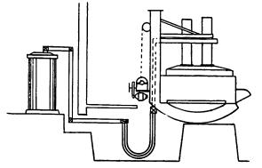
Fig. 1.—Arrangement of Conductors That Limited input to 1500 Kw.
