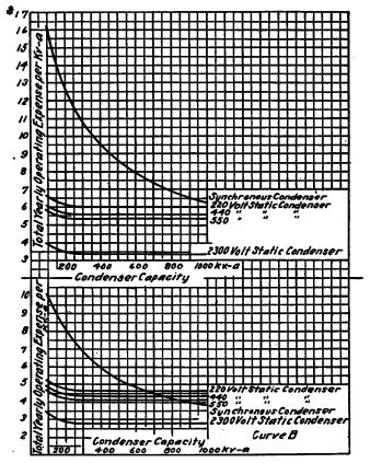
Fig. 5.—Total Yearly Operating Expense per Kv-a./Kv-a. Capacity on Basis of Full-Load Operation 7000 Hrs. per Year.
