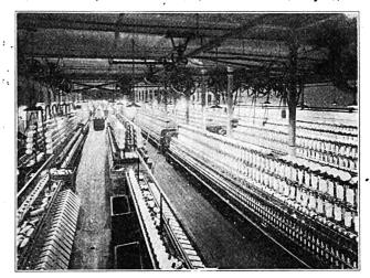
Fig. 5.—View in One of the Spinning Rooms—General Illumination That Floods the Whole Room in Light.
