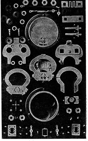
Miniature instrument Disassembled, Showing Parts.
