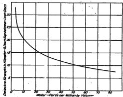
Fig. 2.—Effect of Water on Dielectric Strength of Transformer Oil.
