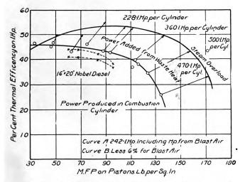
Fig. 2.—Diagram Showing Thermal Efficiency of 13.5 in. by 22 in. Still Engine of the Two-Stroke Opposed Piston Type. Shale Oil Used as Fuel.
