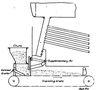
Fig. 1.-Traveling Grate With Producer Hopper.
