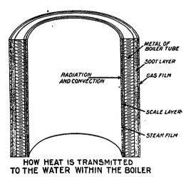
Fig. 1—How Heat is Transmitted to the Water Within a Boller.
