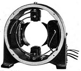
View of Field Frame, Showing Arrangement of Main and Commutating Poles.
