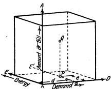
Fig. 9.—Principle Three-Dimensional of Rate Representation.
