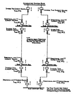
Fig. 2.—Inverser Time Current and Directional Relays as Applied to Ring System.
