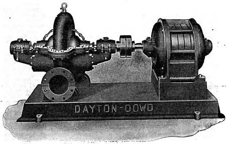
Dayton-Dowd Motor-Driven 8-inch, Single-Stage, Double-Suction Centrifugal Pump.
