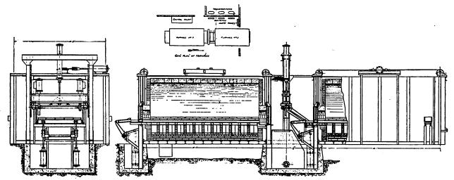
Fig. 4.—Continuous Automatic Two-Furnace, Heat-Treating Equipment for Drawbar Knuckles, Airplane Cranks, Etc., Hydraulically Operated.
