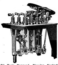
Oil Tank Removed, Showing Contacts and Arcing Shields—By Breaking in a Horizontal Plane the Arcs Do Not Damage Other Parts.
