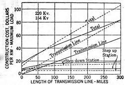
Fig. 2-Economic Comparison of 154-kv. and 220-kv. Transmission-Construction Cost-Seven Lines 154 kv. and Four Lines 220 kv.-500,000 kw. Delivered.
