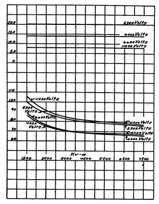
Fig. 3.—Costs of Line, Substation and Connected Installations Per Kv-a. for Various Capacities and Different Voltages.
