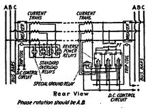
connected in the neutral lead of the current transformers as shown in the accompanying diagram. Then under normal conditions no current flows through the neutral lead of the current transformer bank. But as soon as the ground occurs the unbalanced current flows through this lead and the ground relay and the circuit breaker is opened.
