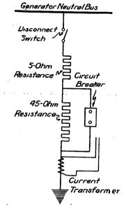
Layout of Resistors, Circuit Breaker and Disconnect Switch to Reduce Current In Neutral.
