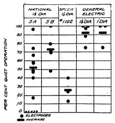
Fig. 11.—Quietness of Operation is Essential When the Operator Has to Listen for Shouted Orders—Many Electrodes of Good Efficiency Were Discarded Because of Hissing—Such Noises Aiso Interfered Greatly with the Listening Devices Auxillary to the Searchilght Equipment.
