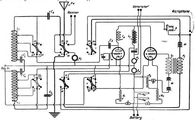
Fig. 6.—Wiring Diagram Showing the Function of the Change-Over Switches.
