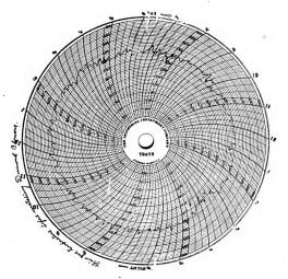
Fig. 3.—Flue Temperatures Before Installing Mechanical Soot Blowers.
