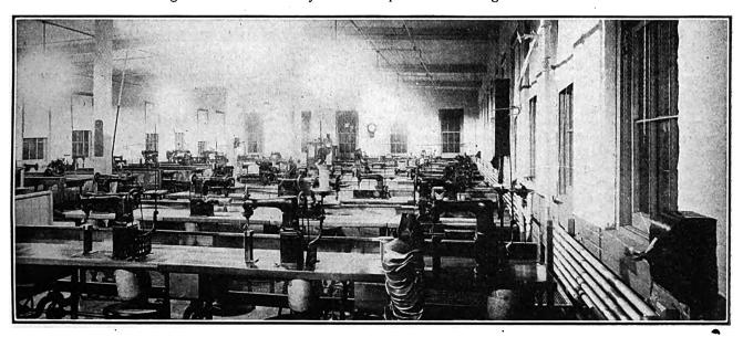
Night View in Sewing Room of a Shoe Factory, Showing That Even the Exacting Work of Sewing Can Be Done Successfully Where Suitable and Yet Highly Efficient General Lighting Is Provided.
