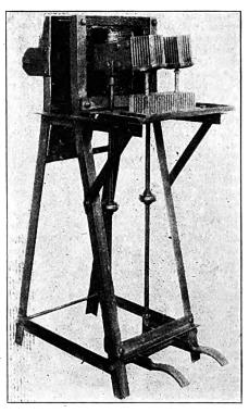
Electric Rivet Heater, Which Does its Work Reliably, Economically and Without Objectionable Features.
