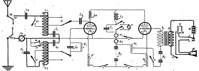
Fig. 2.—The Actual Circuits Used in Practice on the Marconi Transmitter.
