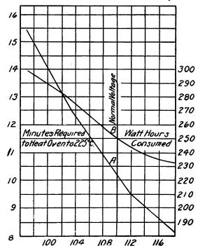
Chart Showing Importance of Maintaining Voltage in Electric Range Operation.
