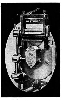
Enlarged View of Berthold Wa Showing the Large One-Piece Enclosing Casting.
