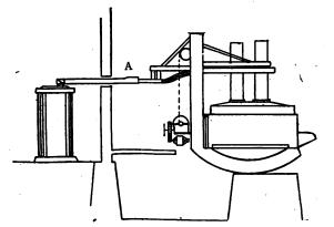
Fig. 2.—Arrangement of Conductors That Enabled Input of 2500 Kw. to be Obtained With Improved Power-Factor.
