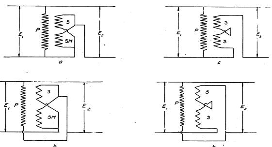
Fig. 1.—Single-Phase Boosting Transf Colls in Parallel.
