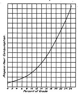
Curve Showing Relation of Ampere-Hour Consumption and Percentage Grade for Electric Truck.
