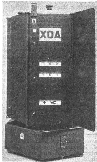
Fig. 1.—Rotating hexagon. Note the large letters above the routine test panels, which are employed in cases where the attitude of the subject under test is in doubt.
