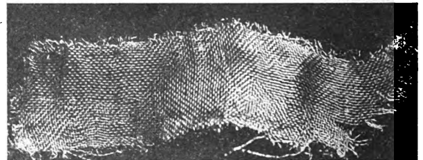
Fig. 6—Portion of tantalum gauze which had been buried in the abdominal wall of an animal for 375 days. The connective tissue has been digested off with pepsin. The original "gun-metal" lustre of the tantalum is undimmed.
