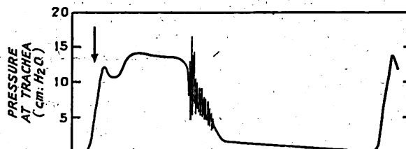
Fig. 11—Pressure record at trachea taken with a condenser manometer, with Radcliffe respiration pump A at 20 respirations a minute. Rapid rise in pressure at start (arrow) of inspiration is a feature of this pump.
