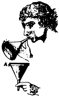
FIG. 15.—The funnel at A has a sheet of india-rubber over the top. When air is sucked out of the funnel the india-rubber curves inwards, owing to the pressure of the air outside.
