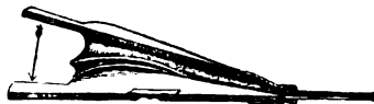
FIG. 14.—When the bellows are being closed the valve is pushed down, and air is forced out of the nozzle.
