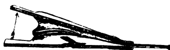
FIG. 13.—When the bellows are being opened the valve rises and air enters.
