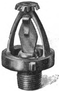
FIG. 7.—Valve of a "Sprinkler" made by Messrs. Mather and Platt. The strip shown in the centre is held together by solder. When a temperature of 155° F. is reached, the solder melts and the valve the strip holds in place opens.
