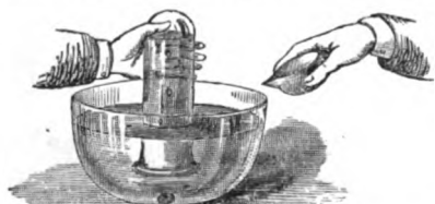
FIG. 12.—Collecting hydrogen from sodium amalgam.
