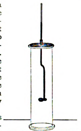
FIG. 9.—Combustion of charcoal in oxygen.
