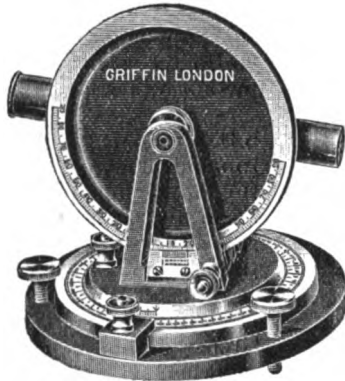
FIG. 2.—A Working Model Theodolite (designed by the Author).
