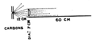
At the lower end two small plano-convex lenses are arranged in such a way as to form a converging lens with a focal length of 10 cm from the lower one.
