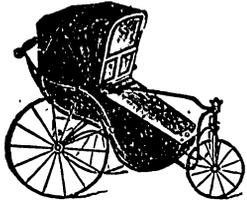
No. 10. — Ward's Victoria Three-Wheel Bath Chair, with leather hood, German shutter, and patent spring front iron, to which shafts for a pony may be attached.
