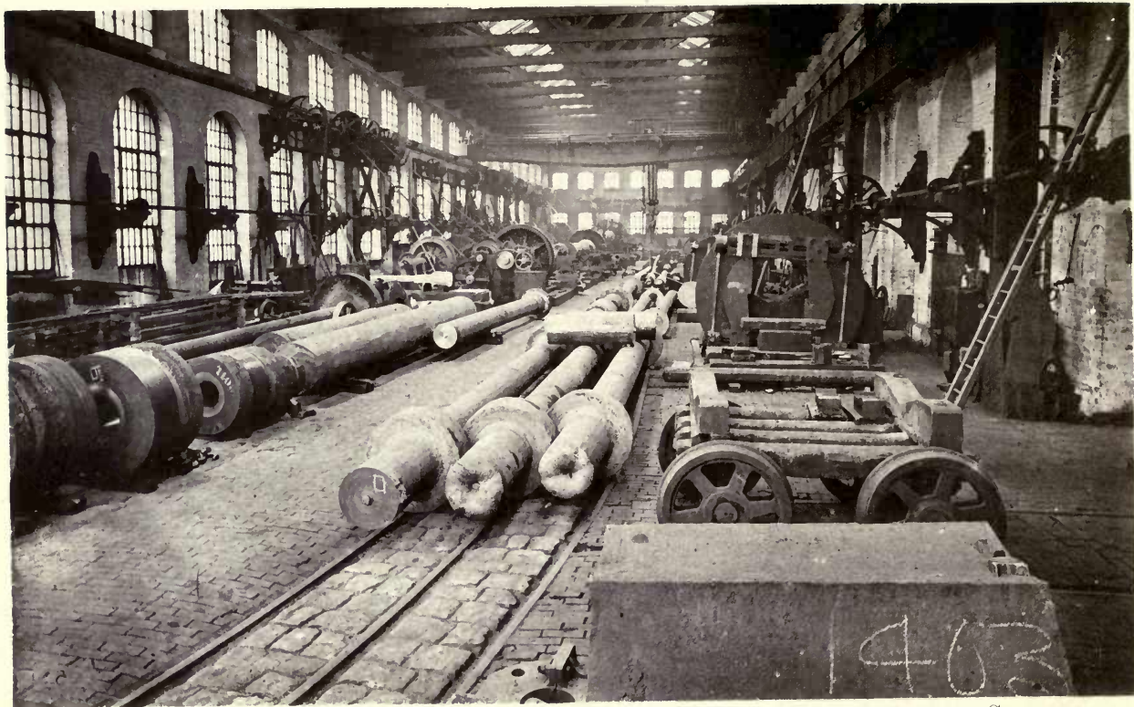
LARGE MACHINE SHOP, 250ft. LONG \times 50ft. WIDE, AT WEST GUN WORKS, SHOWING GUN AND MARINE SHAFT FORGINGS.
