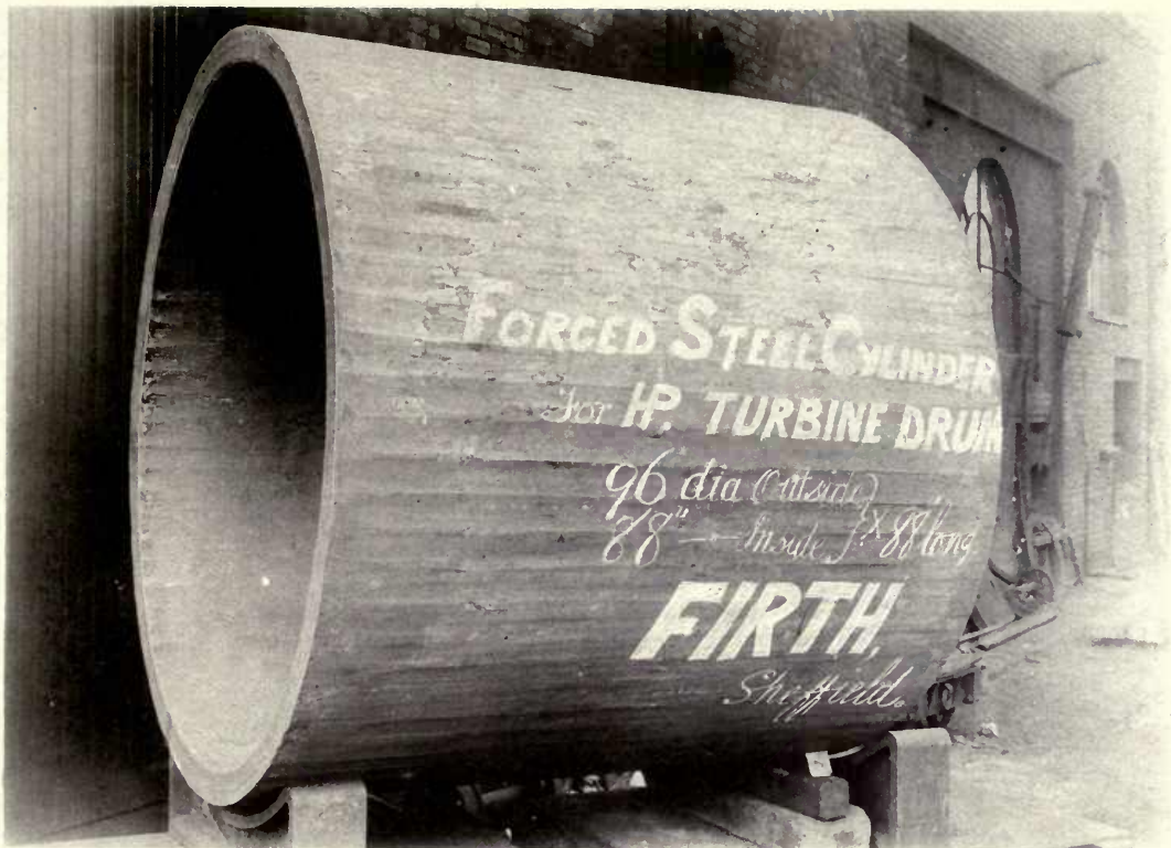
FORGED STEEL CYLINDER FOR H.P. TURBINE DRUM 96in. DIAM. OUTSIDE, 88in. INSIDE, 88in. LONG.
