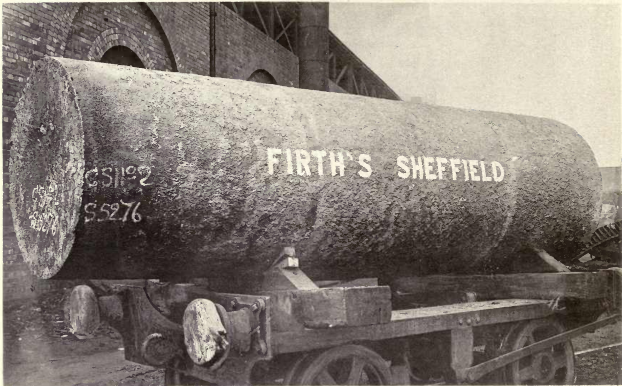
50 TON STEEL INGOT, 53 in. DIAM. × 180 in. LONG.
