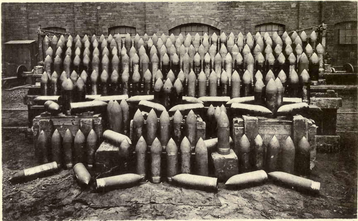
GROUP OF 4.7in. CAST STEEL SHELLS.
