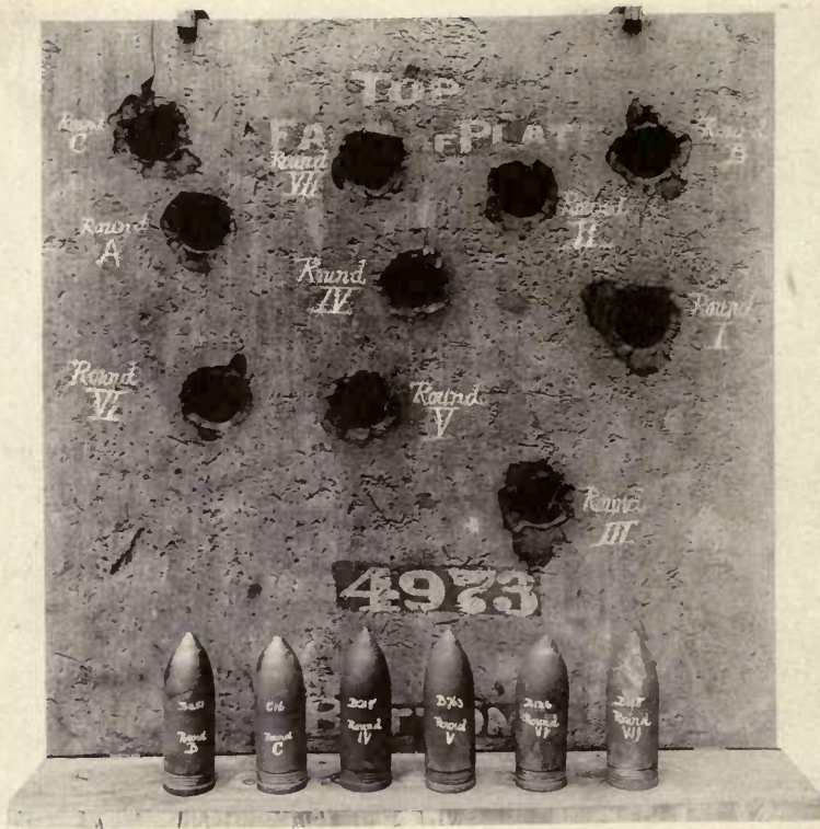
4-7 INCH CAPPED "FIRTH-RENDABLE" A.P. SHELL WITH 4½ K.C. PLATE. SHELL PERFORATED [104] THE PLATE AND WERE RECOVERED WHOLE.
