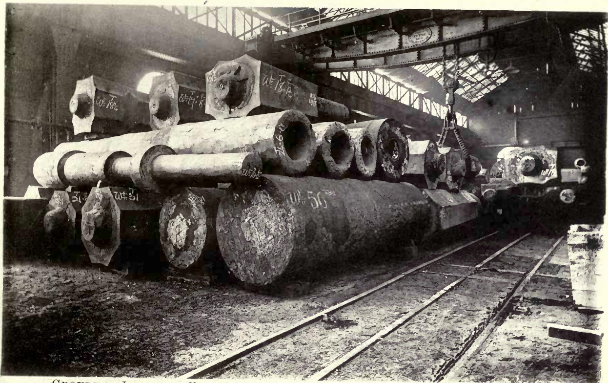
GROUPS OF INGOTS AT EAST GUN WORKS WEIGHING UP TO 56 TONS EACH, ALSO SHOWING 70 TONS, OVERHEAD TRAVELLING CRANE.
