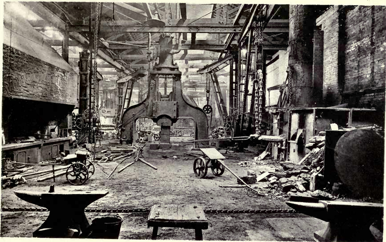
3½ TON STEAM HAMMER, WEST GUN WORKS.
