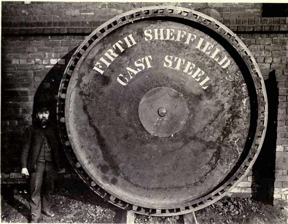
CAST STEEL LOW PRESSURE MARINE PISTON FOR H.M.S. "MONARCH," 9ft. 4in. diam., weight 3\frac{3}{4} ton.
