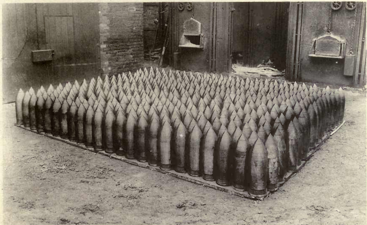
400 7.5in. CAPPED ARMOUR PIERCING SHELL, ACCEPTED AFTER FIRING TRIAL. READY FOR BANDING AND CAPPING. [95]
