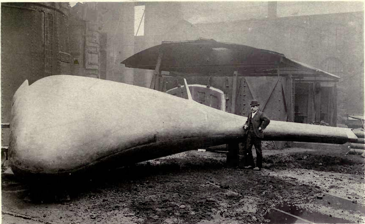
CAST STEEL STEM OR RAM, SUPPLIED TO THE PORTSMOUTH, DEVENPORT & CHATHAM DOCK YARDS FOR H.M.S. "BRITANNIA," "HIBERNIA," AND "AFRICA." [77]
