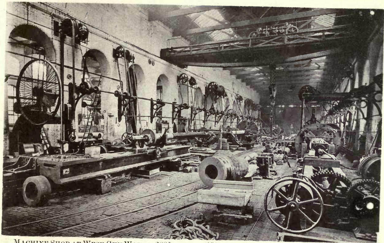
MACHINE SHOP AT WEST GUN WORKS, 200ft. LONG \times 45ft. WIDE, WITH 30 TON TRAVELLING CRANE
