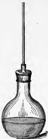
Fig. 43. Flask and Delivery Tube for Ammonia.
