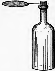
Fig. 106. Wire Ring held by corked Bottle, and supporting a Film of Soap.
