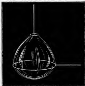
Fig. 108. Soap Bubble supported on Wire Ring, and pulled upwards into a conical shape by means of a Thread.
