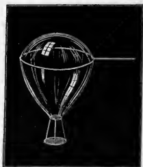
Fig. 109. Soap Bubble supported by Wire Ring and pulled downwards to a conical shape by attached Car and Weights.
